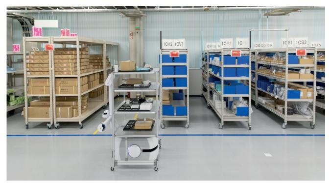
AMRs are one of the most exciting areas for growth in warehouse automation. AMRs assess their environment and move inventory through the facility without direct human supervision, replacing manually operated forklifts. As a result, they eliminate labour intensive and repetitive physical tasks, improving warehouse efficiency, and reducing employee workload.
